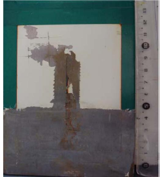
Fig. 3. Photograph of the Reference panel after 641 h in the salt spray chamber.
